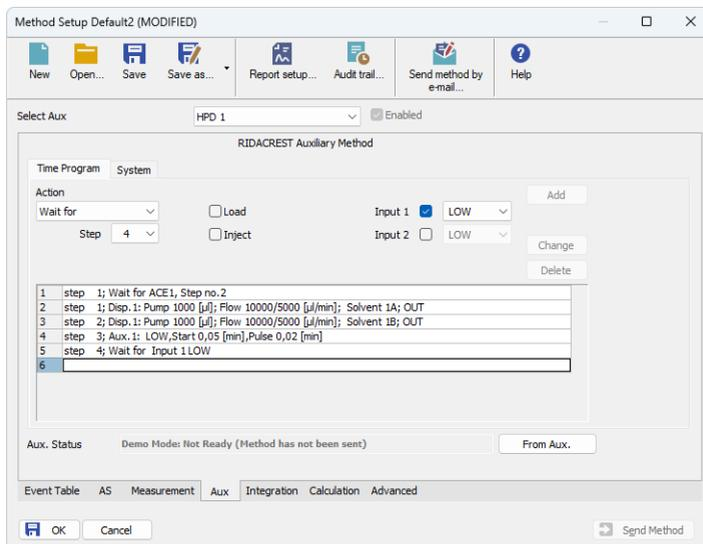
Fig. 8: Method Setup - Aux - Time Program dialog for HPD
