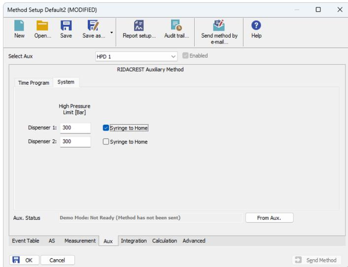
Fig. 9: Method Setup - Aux - System dialog for HPD
