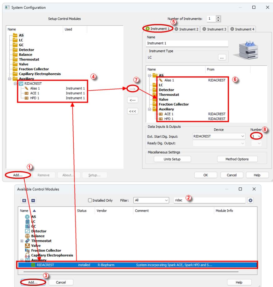
Fig. 3: System Configuration
