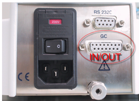
Fig. 3: Autosampler IN/OUT connector
