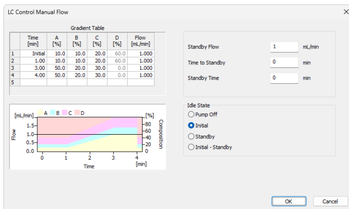
Fig. 14: LC Control Manual Flow dialog
