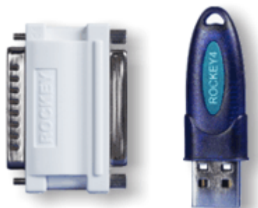
Rockey LPT and USB hardware keys (dongles)
