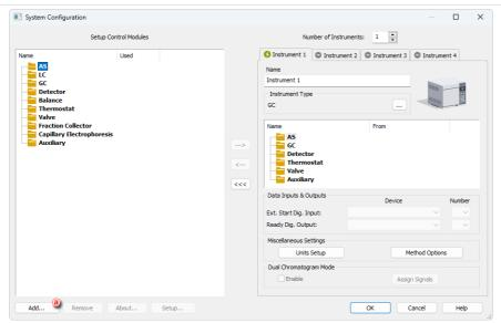
2. If the device you want to add is not in the list, click on *Add* ⓐ and the *Available Control Modules* dialog will open. Here, you can filter the list by typing some text in the filter field ⓑ.
