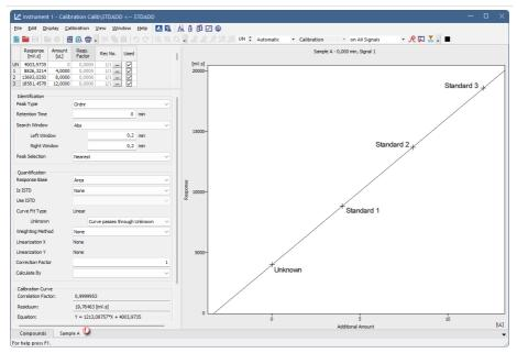
14. Open chromatogram of the desired unknown sample. The Result Table now contains amount of the unknown sample, calculated using Standard Addition.
