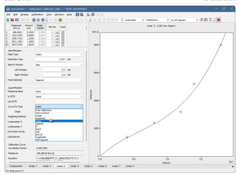
As you can see, changing the *Curve Fit Type* from *Linear* to *Cubic* increased the *Correlation Factor* from 0.954 to 0.992.
