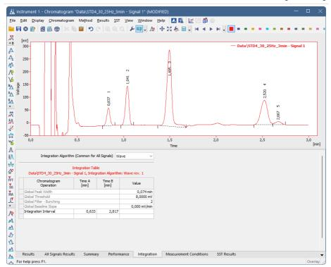
6. (Optional) Set the *Detect Negative* parameter. This setting has two potential uses: firstly, it can be used when you want to integrate negative peaks; secondly, it may help when the signal has inconsistencies such as dips. This will prevent the integration algorithm from placing peak starts/ends into them.
