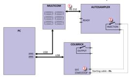
Fig. 11: Wiring of the autosampler with AS Control module + A/D converter
