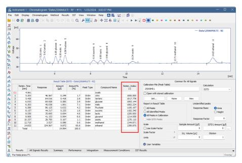
The *Unretained Peak Time* can be used for adjusting the retention times for more precise calculation of retention indexes:
