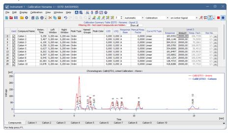
Note: It is possible to review calibration curves for each compound on the respective tabs of individual compounds. Notice that calibration curve are displayed only for valid signal (When filtering is enabled tabs of individual compounds are displayed only on signal where they are used). Signal selection is located in right upper corner of the Calibration Window.
