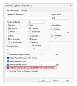
3. The *Unretained Peak Time* may be entered in the *Method Setup - Advanced* tab, or directly in the chromatogram on the *Performance* tab.
