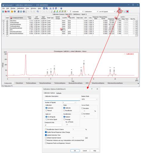
Now, the first calibration level is set. Continue as usual to set the remaining calibration levels using the measured calibration standards (as shown in <u>Adding</u> <u>a new calibration level</u>). Enter the ISTD amounts according to the mode you plan to work in.
