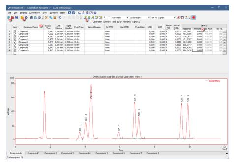
4. Select the Save As option. In the Save As dialog check the Clear Responses checkbox and save the calibration under a new name.
