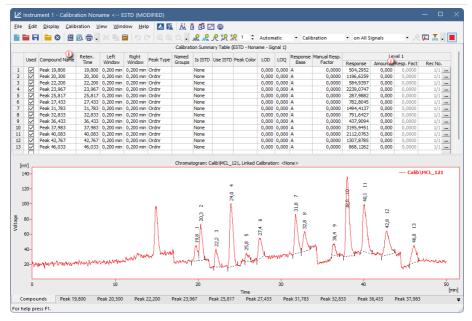
If you selected Manual calibration: Fill in the Amount, the Compound Name and set any other parameters related to the peak on the Calibration - Add Peak window. This window will open once for each one of the peaks processed.
