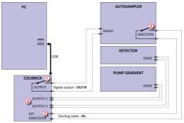
Fig. 6: Wiring of the autosampler in an LC set without the AS Control module
