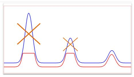
It is possible to indicate that a signal has reached a value out of the detector range via scheduling an event in the Event table. Such event needs to be triggered by the signal reaching a specific value, that is right below the detector maximum.
