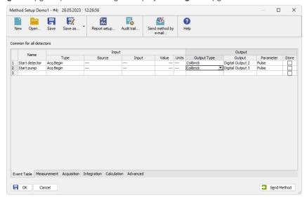
Fig. 8: Event Table for starting detector and pump from Clarity
