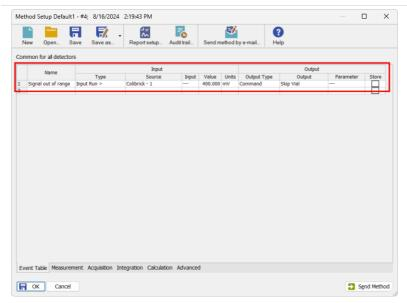
Once the entered input value is surpassed, the specified output event is triggered. Suitable output events also include alarm activation, close a contact, etc.
