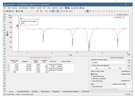
Note the two vertical guidelines marking the beginning and end of the peak. After finishing the operation new peak is added ©.
