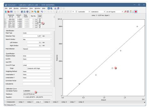
As you can see, excluding the incorrectly measured calibration point resulted in more accurate calibration.
