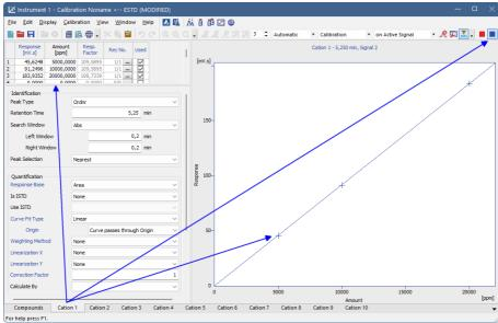
19. When calibration is finished do not forget to save it using select *File - Save* or click on ...
