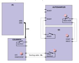
Fig. 9: Wiring of the autosampler in Passive Sequence
