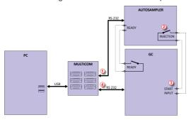
Fig. 13: Wiring of the autosampler with AS Control module and digital acquisition
