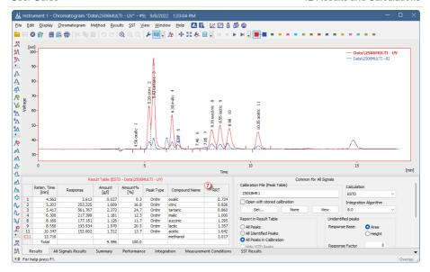
Note: You can do a quick check that the calculation is correct: look at the malic compound, the RRT should be 1.
