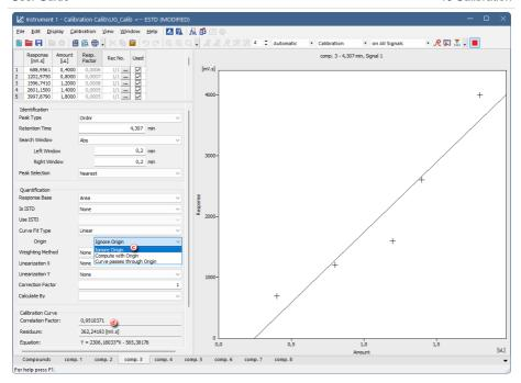
As you can see from the *Correlation factor* ① values, changing the *Origin* setting from the *Curve Passes through Origin* to *Compute with Origin* improved the curve fit. However, the option *Ignore Origin* has proved to be the best match for the used detector.
