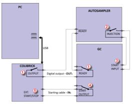
Fig. 2: Wiring of the autosampler - variant A
