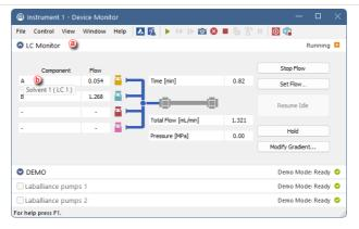
Further commands are available for selected pumps (typically those controlled by **Clarity** in real time). They are enabled only during runs with a gradient program.
