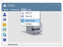
2. After logging in to the Instrument, new windows open in tablet layout. *Instrument window* is positioned to the left side of the monitor, other windows open on top of each other and fill the remaining space on the monitor.
