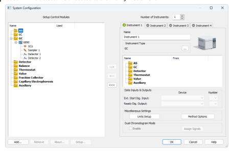
Fig. 24: Detector not allocated to the Instrument
