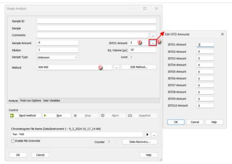
The sequence analysis setup is analogous to the single analysis. The ISTD2–ISTD10 amount columns are not shown by default and can be added via the *Edit - Setup columns...* dialog.
