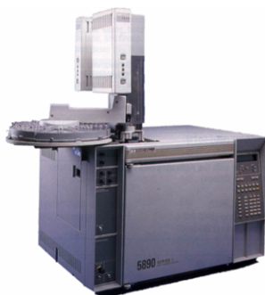
Fig. 1: Agilent (HP) 5890 with an autosampler
