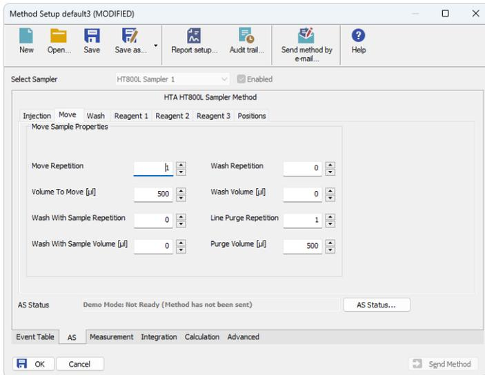
Fig. 7: Method Setup - AS - Move
