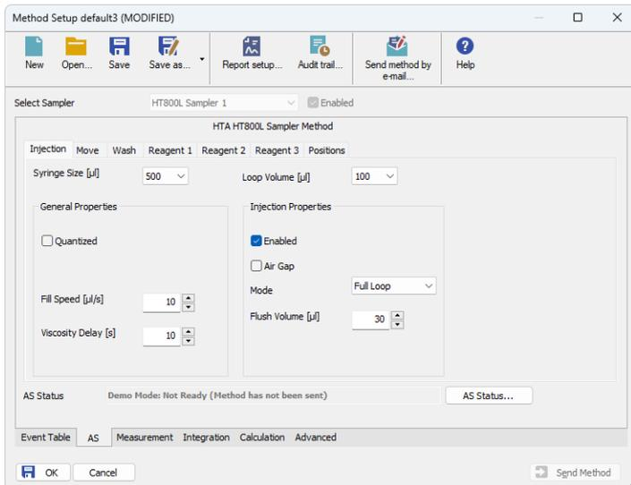
Fig. 6: Method Setup - AS - Injection
