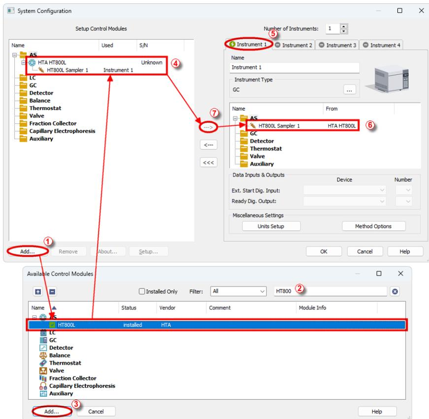
Fig. 4: System Configuration
