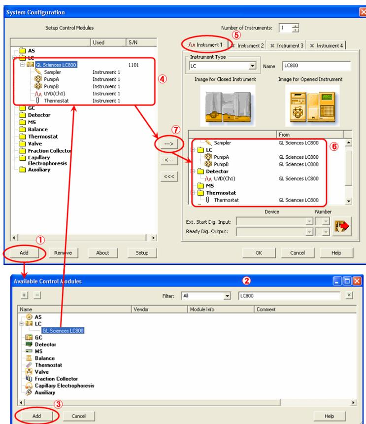
Fig 2: System Configuration
