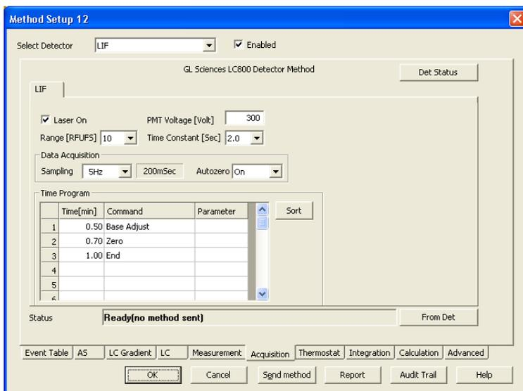
Fig 18: Method Setup - Acquisition - LIF
