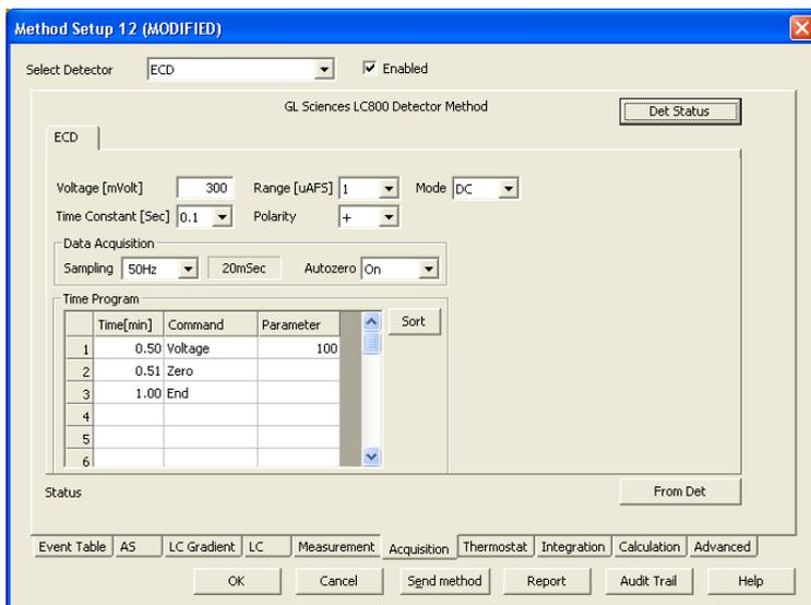
Fig 19: Method Setup - Acquisition - ECD
