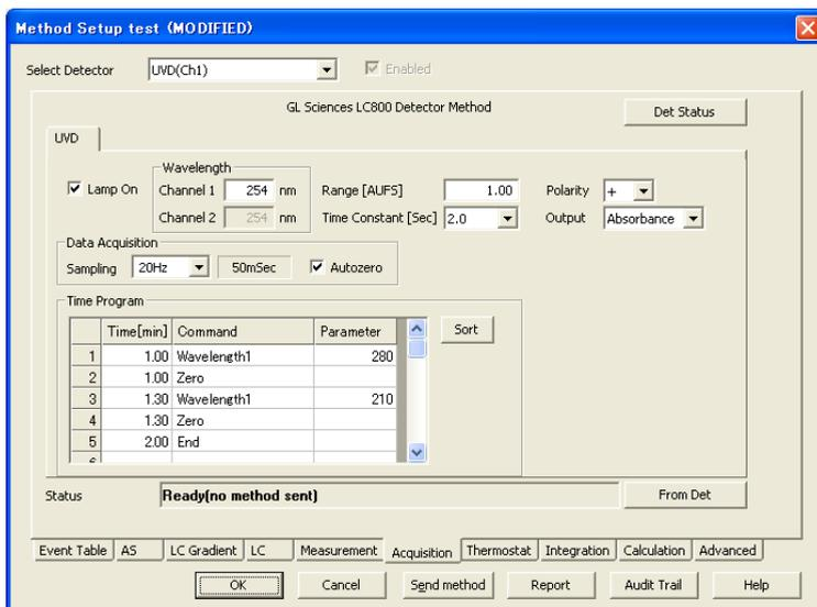
Fig 16: Method Setup - Acquisition - UVD
