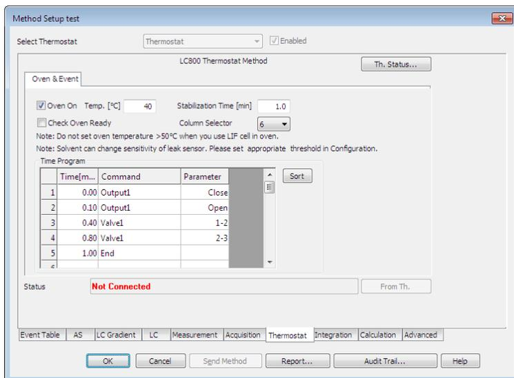
Fig 34: Method Setup - Thermostat
