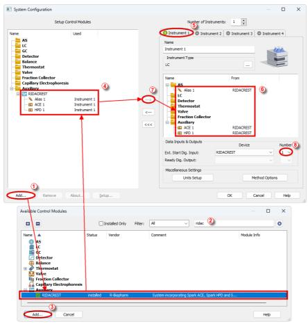
Fig. 3: System Configuration
