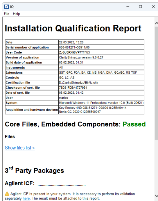
Fig. 8: IQ Report with ICF installation present
