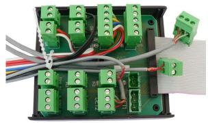
The individual connectors can be taken out, and LEDs indicate the state of the inputs/outputs
