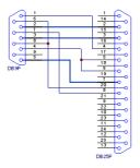
Fig. 2: Serial cross DB9F - DB25F cable
