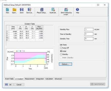
Fig. 5: Method Setup - LC Gradient
