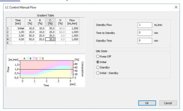
Fig. 14: LC Control Manual Flow dialog
